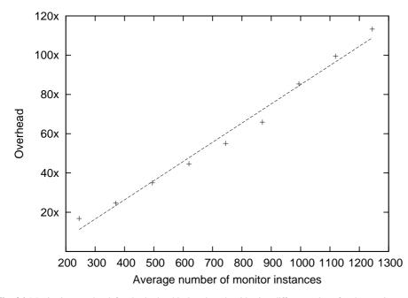
Fig. 26 Monitoring overhead for the hash table benchmark with nine different values for the maximum table size. We calculate the number of monitor instances, shown on the x-axis, as the average number of instances that exist when a tracecut event is monitored. As with our bzip2 benchmark in Section 4.2, we obtained performance numbers by comparing the average execution time of the benchmark with and without monitoring, using ten runs for each.
