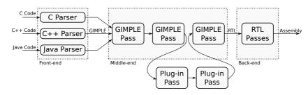
Fig. 1 A simplified view of the GCC compilation process.
