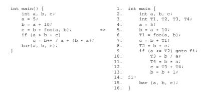
Fig. 2 Sample C program (left) and corresponding GIMPLE representation (right)
