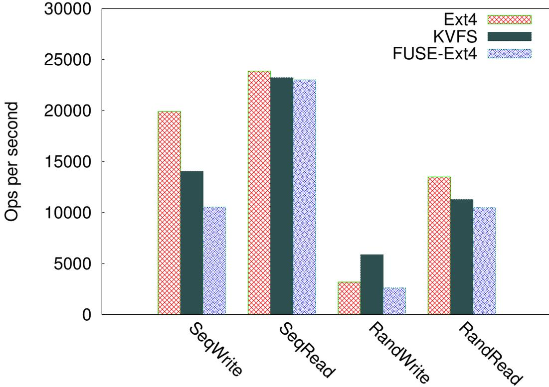
Figure 4.4: Filebench results for micro-benchmark workloads on SSD
