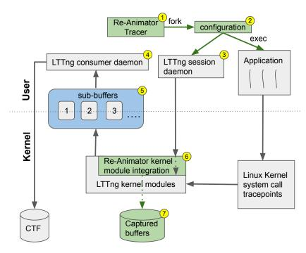
Figure 4.1: LTTng architecture using Linux kernel tracepoints. Green boxes denote our additions or changes. Our wrapper (1) launches the LTTng configurator (2), which invokes an LTTng session daemon (3) to control the operation and the consumer daemon (4) to collect events. LTTng tracepoints place events into sub-buffers (5) and invoke Re-Animator, which collects data buffers and writes them to a separate disk file (7).
