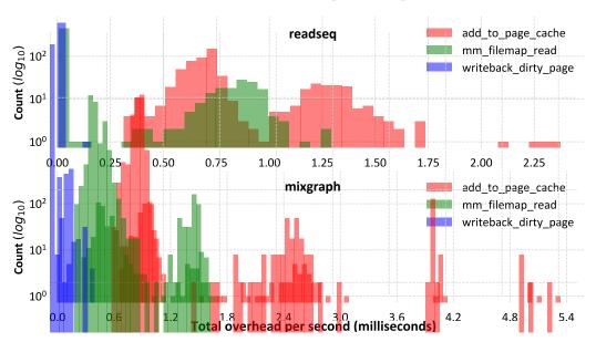
Figure 5.7: Distribution of total data collection overhead (milliseconds) in every second when readseq and mixgraph workloads are running.
