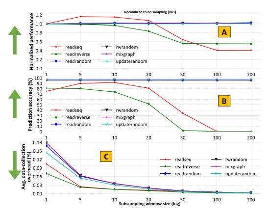
Figure 5.6: Performance (A), prediction accuracy (B) and CPU overheads (C) in seven different subsampling window sizes for the per-disk readahead neural network. Upward green arrows denote that higher is better.
