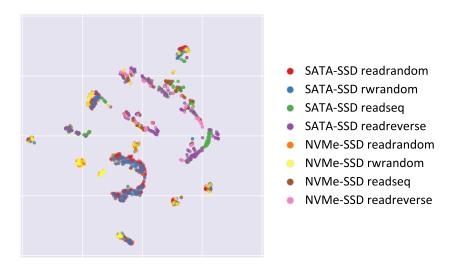
Figure 5.4: t-SNE visualization of readahead normalized features that are generated from both NVMe-SSD and SATA-SSD traces. Axes are intentionally omitted because the dimensions are generated by t-SNE and do not represent any specific data.
