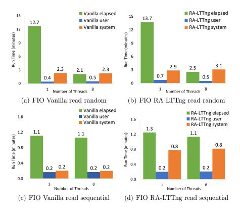
Figure 4.2: FIO random and sequential read times in minutes (elapsed, user, and system). Vanilla denotes FIO without tracing; RA-LTTng denotes FIO with full tracing enabled. Note that the Y-axis scales differ between the random and sequential pairs of figures.
