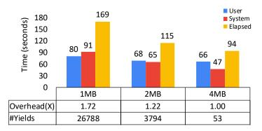
Figure 4.5: RA-LTTng blocking-mode overheads for tracing LevelDB db\_bench with its default database configuration. We used 3 different RA-LTTng sub-buffer sizes (4MB, 2MB, and 1MB); we show user, system, and elapsed times for each experiment. The table below also shows the elapsed time overheads relative to the 4MB baseline and the number of yield calls executed.
