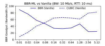
Figure 6.1: Bandwidth sharing percentages when Cubic and BBR flows run concurrently under different bottleneck router buffer size configurations in BDP.
