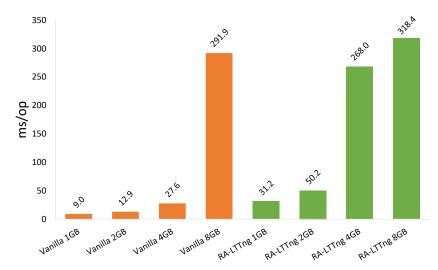
Figure 4.4: LevelDB read-random latency for different-sized databases (in milliseconds per operation).
