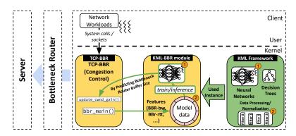
Figure 6.2: KML BBR Architecture
