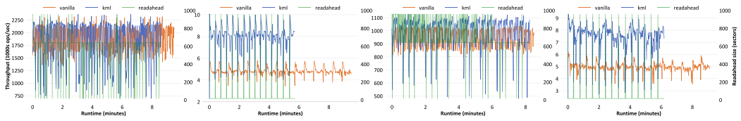
Fig. 8. Running four back-to-back RocksDB workloads in order from left to right: readsequential, readrandom, readreverse, then mixgraph. Here, we started with the default readahead value; thereafter, the last value set in one workload was the one used in the next run. For each of the four graphs, we show their Y axes (throughput, different scales). The readahead value is shown as the Y2 axis for the rightmost graph (d) and is common for all four. Each workload ran 15–50 times in a row, to ensure we ran it long enough to observe patterns of mis/prediction and reach steady state. Periodic spikes that we observed in readrandom and mixgraph denote the experiments’ starting points because of multiple iterations of benchmarks. Again, we see KML adapting, picking optimal readahead values, occasionally mis-predicting but quickly recovering, hence overall throughput was better.
