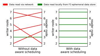
Figure 5: Impact of data aware scheduling. Each line connects a writer with its corresponding reader, with the numbers along each side showing what node in the cluster the writer or reader ran on. Red lines indicate that the reader needed to transfer its file from the writer node via a network transfer. Green lines indicate that the reader and writer ran on the same node and the file was read from F3's local ephemeral data store, with no network transfer was needed.
