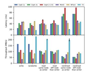
Figure 6: Mean latencies and bandwidths of Ceph, NFS, MinIO, and F3. "Ceph 1×" and "Ceph 3×" are configured with 1× and 3× replication, respectively. "Ceph 2-1 EC" uses erasure coding (data split into two data chunks and one coding chunk). F3 was layered on top of an unreplicated CephFS volume.
