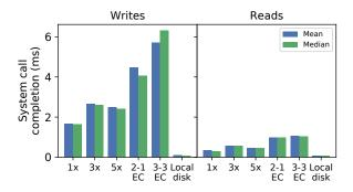
Figure 3: Mean and median system call latencies for different configurations of storage system.  $1\times$ ,  $3\times$ , and  $5\times$  refer to the degree of replication; 2-1 and 3-3 EC refer to the erasure coding configuration (2 data and 1 coding chunk, and 3 data and 3 coding chunks, respectively).
