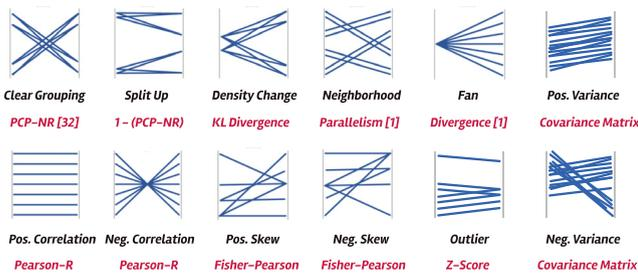
Fig. 3. Properties and their corresponding line patterns detectable in PC-Expo. Blumenschein *et al.* [7] proposed these line patterns and related them to common analytical tasks. Below, in red, each analytical task is the method we have used in PC-Expo to detect the corresponding patterns locally in the data.
