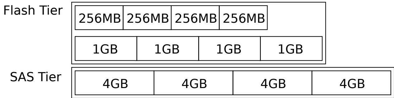
Figure 5.4: Configuration of re-insertion caching benchmark: Storage is divided into two tiers, Flash and SAS (magnetic disk).
